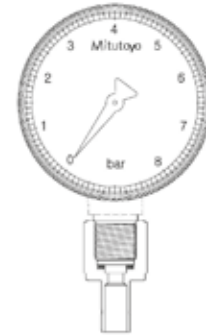
Gauge Adapter helps set a gauge-facing direction.
